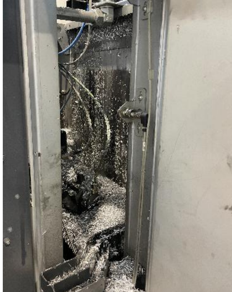
Gripper Drive Compartment Filled with Chips
