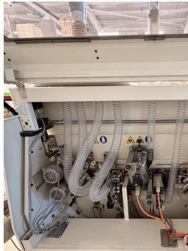
SMC edging machine replace pipes of duster system
